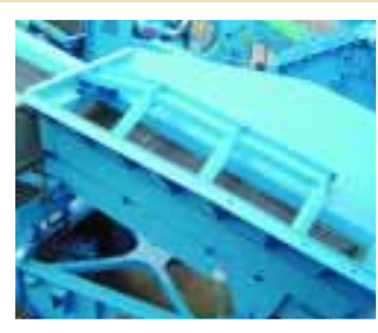
▲ FEED HOPPER Heavy duty Hardox feed hopper with impact channels to protect feed belt.
