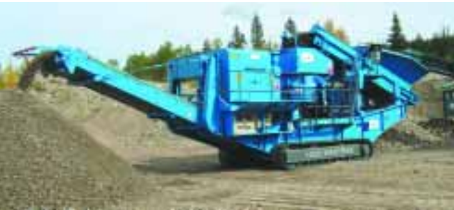
▲ HIGH CAPACITIES The 1300 Maxtrak is capable of capacities up to 350 mtpg depending on the type of material.
