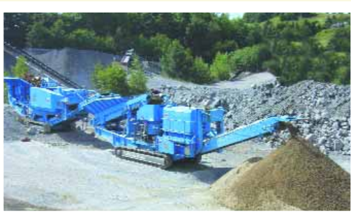
▲ The 1000 Maxtrak has been designed to maximise throughput, reduction and product shape in a wide range of quarrying applications.
