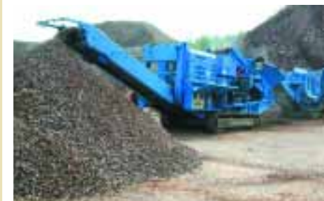
▲ 1165 Premiertrak working with a 1000 Maxtrak to produce 40mm sub-base on a basalt application.
