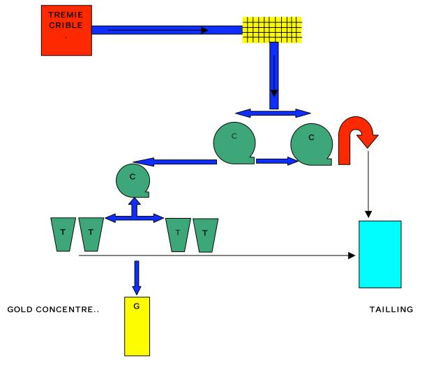
PROCESS PLANT. ALLUVIA GOLD. SCPM. METHODE PAR GRAVITE DENSIMETRIE.
